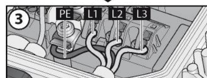
Fig. 3: Connecting wires to terminals
