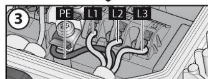
Fig. 3: Connecting wires to terminals
