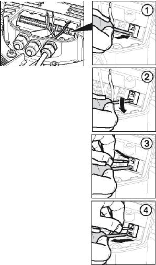
Fig. 2: Connecting wires to terminals
