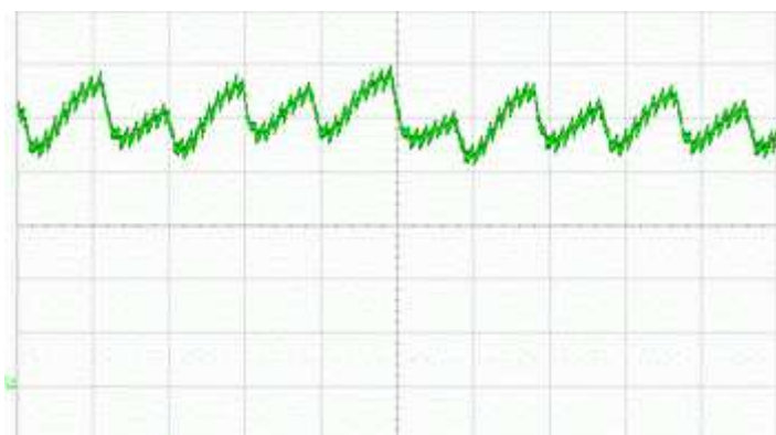
Running current @ 24 V ( I = 500\text{mA/div} ; t = 500\text{us/div} )
