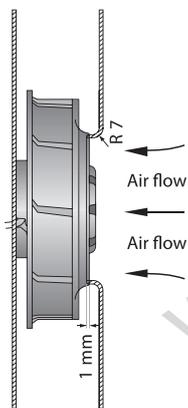
The air flow and sound level of the centrifugal fans without external housing depend on their individual installation conditions.
