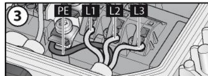
Fig. 2: Connecting wires to terminals
