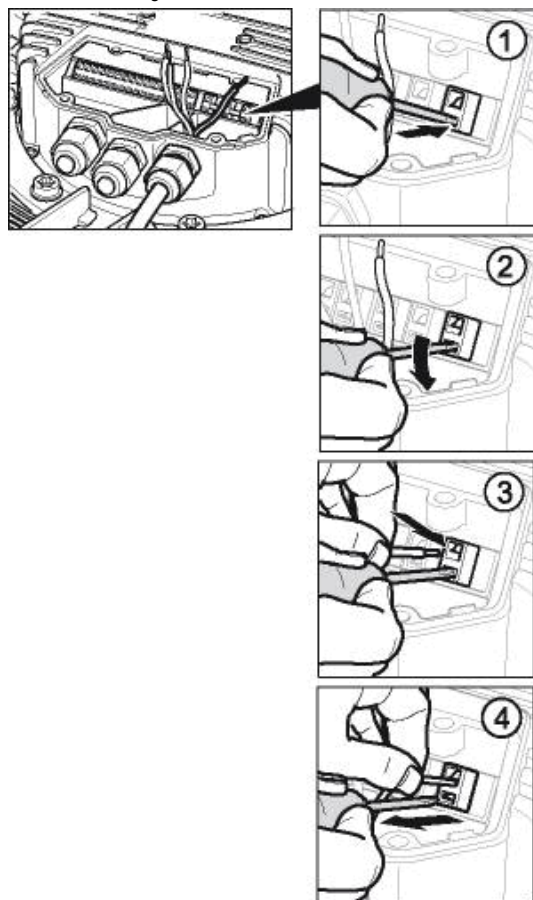
Fig. 2: Connecting wires to terminals
