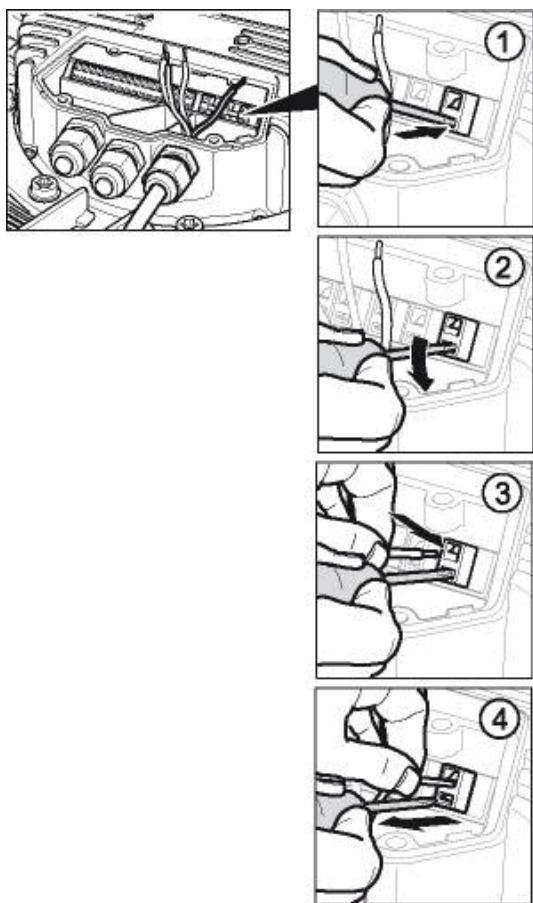
Fig. 2: Connecting wires to terminals
